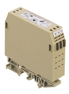
On-delay timing relay, time range: 3 s to 30 s, Screw connection, Mounting type: Mounting rail TS 35, 1 CO contact, Supply voltage: 24 VAC/DC
