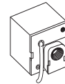
Example of a tube with external diameter of \phi 4 and internal diameter of \phi 2.5
