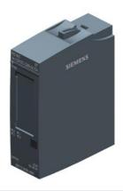
SIMATIC ET 200SP, Relay module, RQ NO 4x 120V DC..230VAC/5A ST. 4 normally open contacts, isolated contacts, packing unit: 1 piece, fits to BU-type B0 and B1, Colour Code CC40, substitute value output, module diagnostics for: supply voltage
