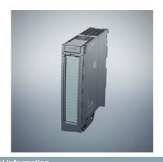
SIMATIC S7-1500, Digital output module DQ 16x 230 V AC/2A ST; Relay 16 channels in groups of 2; 4 A per group; switching cycle counter for integrated relay, diagnostics; substitute value: front connector (screw terminals or push-in) order separately
