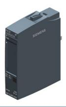
SIMATIC ET 200SP, Signal relay module, RQ CO 4x 24V DC/2A ST, 4 changeover contacts, isolated contacts, packing unit: 1 piece, fits to BU-type A0, Colour Code CC00, substitute value output, module diagnostics for: supply voltage
