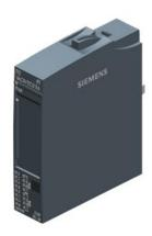
SIMATIC ET 200SP, Digital output module, DQ 16x 24V DC/0,5A Standard, Source output (PNP,P-switching) Packing unit: 1 piece, fits to BU-type A0, Colour Code CC00, substitute value output, module diagnostics for: short-circuit to L+ and ground, wire break, supply voltage
