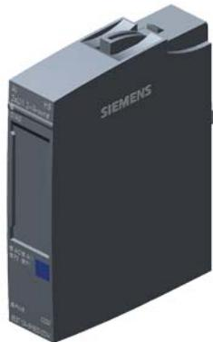
SIMATIC ET 200SP, Analog input module, AI 2x U/I 2-/4-wire High Speed, suitable for BU type A0, A1, Color code CC00, channel diagnostics, 16 bit, +/-0.3%
