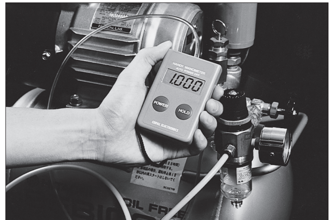
▲ Measurement of source pressure from a compressor.
